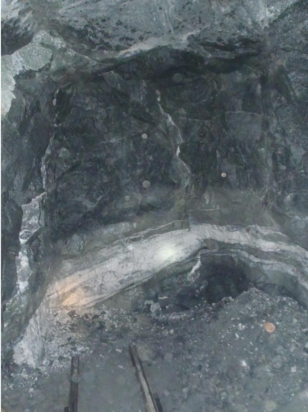
Photo 2: McNally's Reef Development Heading on 27.02.2019 with quartz reef in the position interpreted from diamond drilling
