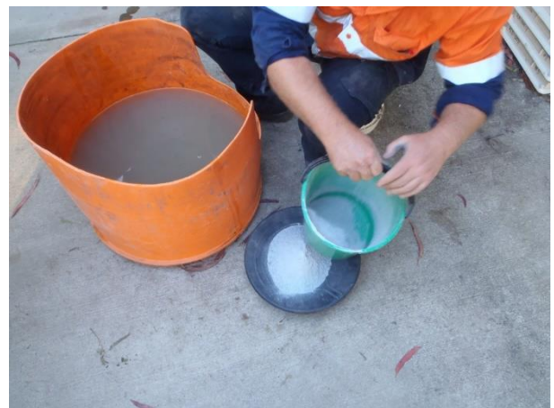
Photo 5. Crushed rock being prepared to be panned for visible gold and sulphides for immediate decision making. Raw duplicate samples are sent to a commercial laboratory for confirmation
