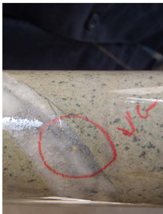
Plate 2 - Visible gold in a 2 cm stockwork vein in highly altered diorite dyke at 12.9 metres down hole ROD 012A
