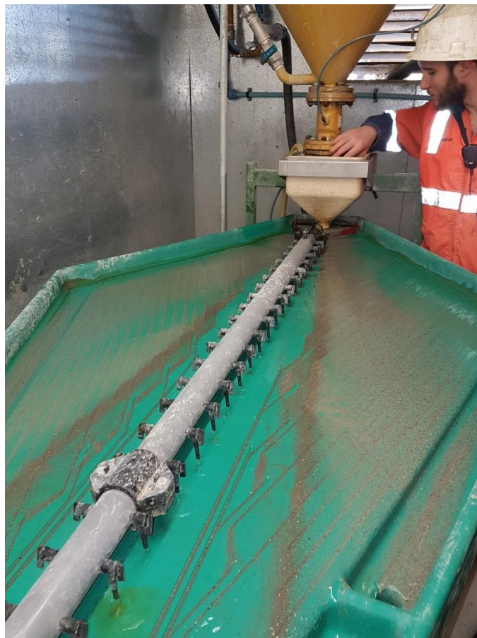
Photo 3. Gold room: Gold concentrate after first pass on the gravity separation table
