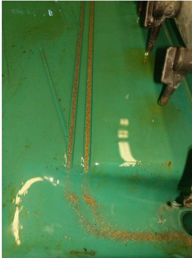
Photo 2. Gold room: Gold concentrate after multiple passes on the gravity separation table
