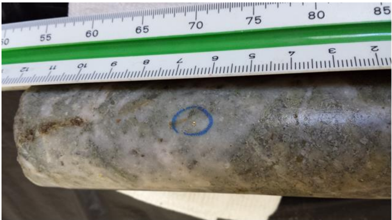
Photo 2. Visible gold in altered dyke in drillhole L7016, at 44.15 m down hole.
