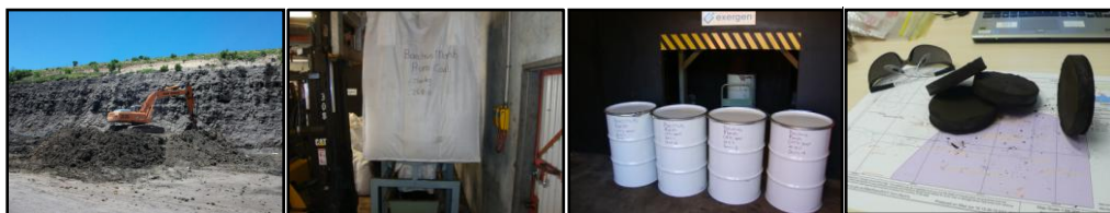
Figure 1: ROM coal (56.7% moisture), CHTD Pilot Plant Processing and resulting briquettes (9.5% moisture).
