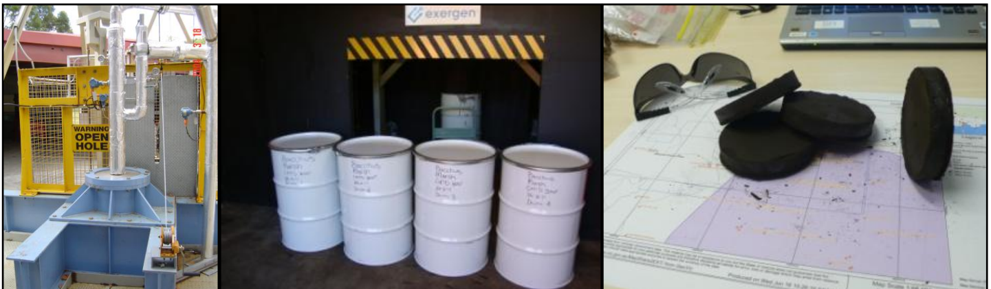
Figure 9: CHTD Pilot Plant Processing of Bacchus Marsh coal (56.7% moist) and resulting briquettes (9.5% moist).
